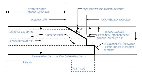
Safety Edge Dimensions for Asphalt Pavement (New Construction >/= 6" thickness)
