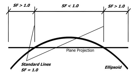
**Figure 9 –** Unlike the elevation factor (which is less than 1.0 throughout West Virginia), the scale factor can be less than or greater than 1, depending upon whether the plane is above or below the ellipsoid surface as shown in the cross section above.
