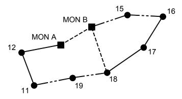
**Figure 4 –** Individual observations in the control network are shown as different linetypes.
