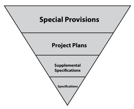
Project plans or plan notes should not be used to change specifications. The procedure outlined in this Design Directive should be utilized when this is necessary.
