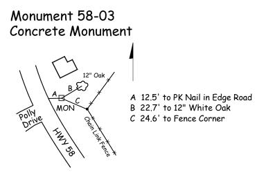
**Figure 5 –** A sketch of the monument should include the major features found in the landscape near the area of the monument and at least three distances to easily identifiable points.
