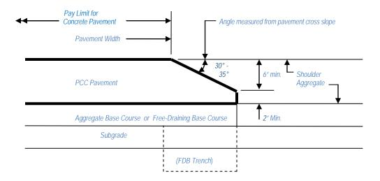
Safety Edge Dimensions for Concrete Pavement (New Construction)
