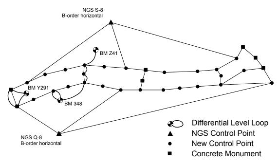
**Figure 2 –** While the minimum requirements are met for the number of horizontal and vertical control points in the network, the location of the vertical ties would be expected to provide less accurate elevations for the eastern limits of the project.
