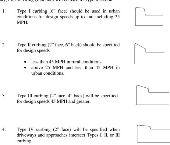
Caution should be exercised in the use of curbs on rural highways. Curbs should be omitted on rural highways when the same objective can be attained by other acceptable means. In general, curb is not desirable on high speed roadways, If curbing must be used, only Type III will be specified for design speeds 45 MPH and greater.
