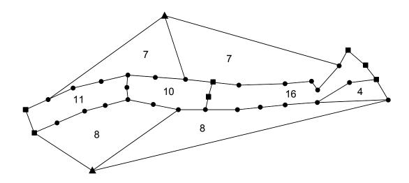
**Figure 3 –** The number of independent baselines in each of the closed loops is shown in the network above. The rules for construction of a control network are violated as 16 baselines comprise the loop found in the right half of the network.
