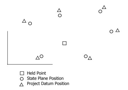
**Figure 8 –** The new positions of the points on the project datum reflect a stretch outward from the held point. In this case a point near the center of the project was held fixed.
