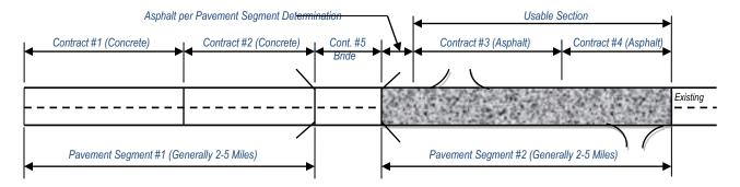
Figure 1. Illustration of contracts within pavement segments
