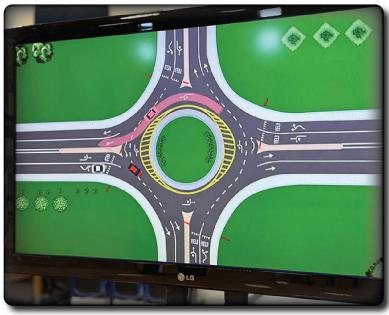
The proposal is for a boulevard style roadway from Great Teays Boulevard to Scott Lane with roundabouts at key intersections to ease congestion. There would also be a six foot bike lane and five foot sidewalk in each direction. The center island would be eight feet wide and could be used for plantings and lighting.
