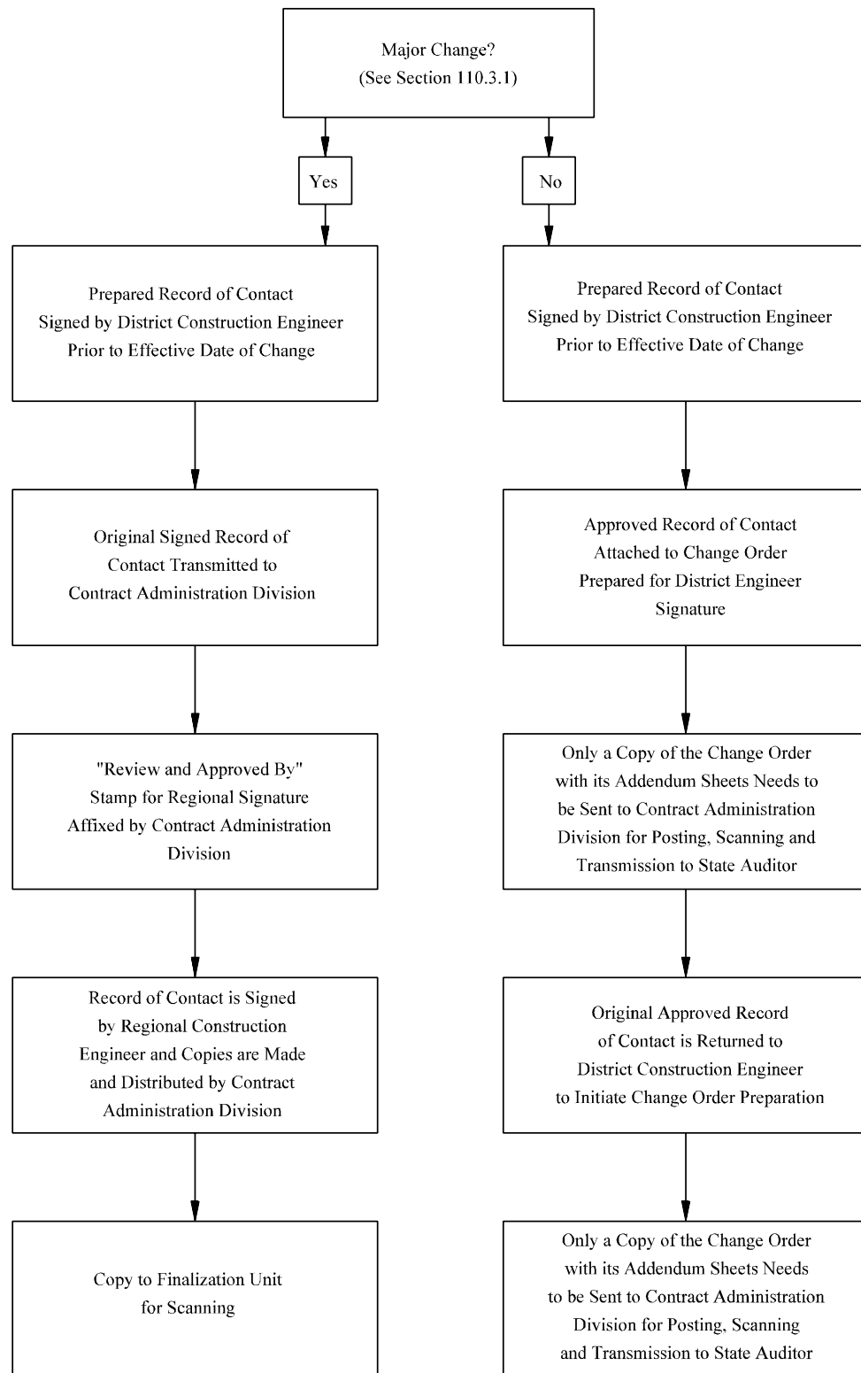
PROCESSING FLOWCHART FOR STATE FUNDED AND EXEMPT FEDERAL-AID PROJECTS Figure 110B
