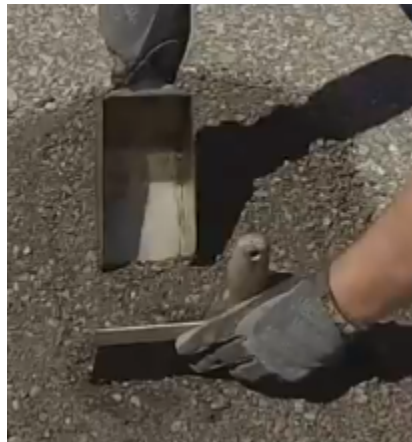
Figure 40 - Roadway Scoop Sampling
