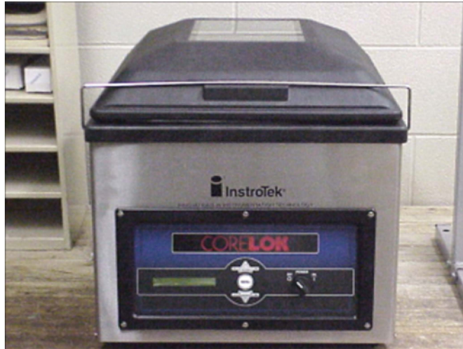
Figure 48 - Vacuuming Sealer for AASHTO T 331
